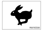
When this lamp turned ON, the machine travel high speed.
